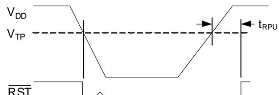
A watchdog timer can also be used to drive an active reset signal. The watchdog is a free-running programmable timer. The timeout period can be software programmed from 100 ms to 3
