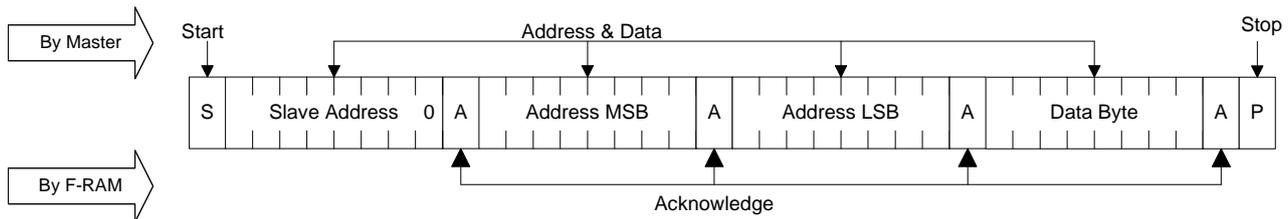
Figure 18. Multi-Byte Write
