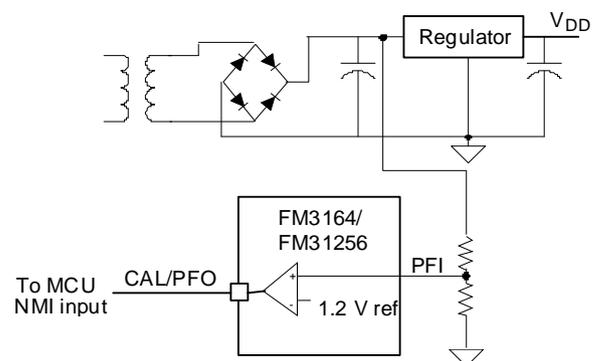
The voltage on the PFI input pin is compared to an onboard 1.2 V reference. When the PFI input voltage drops below this threshold, the comparator will drive the CAL/PFO pin to a LOW state. The comparator has 100 mV (max) of hysteresis to reduce noise sensitivity, only for a rising PFI signal. For a falling PFI edge, there is no hysteresis.
