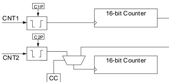
The control bits for event counting are located in register 0Ch. Counter 1 Polarity is bit C1P, bit 0; Counter 2 Polarity is C2P, bit 1; the Cascade Control is CC, bit 2; and the Read Counter bit is RC, bit 3.
