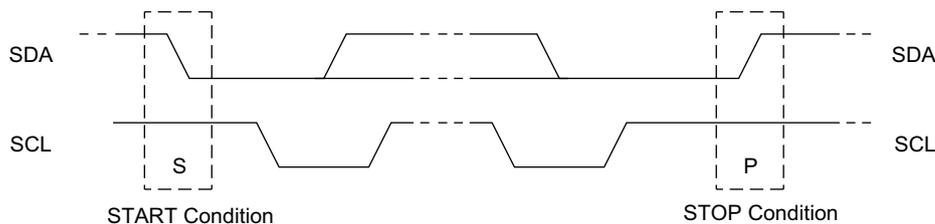
Figure 13. Data Transfer on the I<sup>2</sup>C Bus
